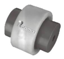
Flexitech Nylon gear Coupling is curved tooth coupling consisting of two steel crowned teeth hubs which are connected with nylon (Polyamide) internally toothed sleeve. These materials are resistant to all the usual commercial lubricants and hydraulic fluids.
